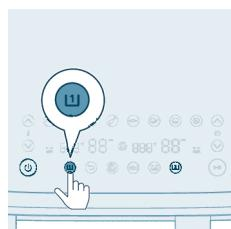
9 Press the temperature up/down button and time up/down button to choose the needed time and temperature.
