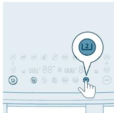
**11** Press the temperature up/down button and time up/down button to choose the needed time and temperature.
