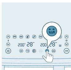
**13** Press the Start/Stop button to start the cooking process.
