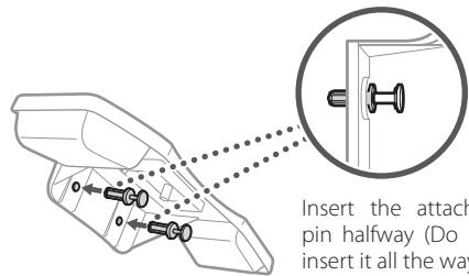
Insert the attached pin halfway (Do not insert it all the way in here).
