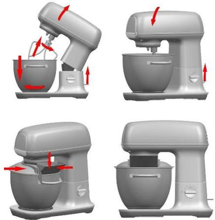
Your accessories are equipped with a system for adjusting the height above the bottom of the bowl for optimum results. Depending on the nature of the ingredients, the bowl (7) with its cover can be used to prepare up to 1,5 kg of dough.
