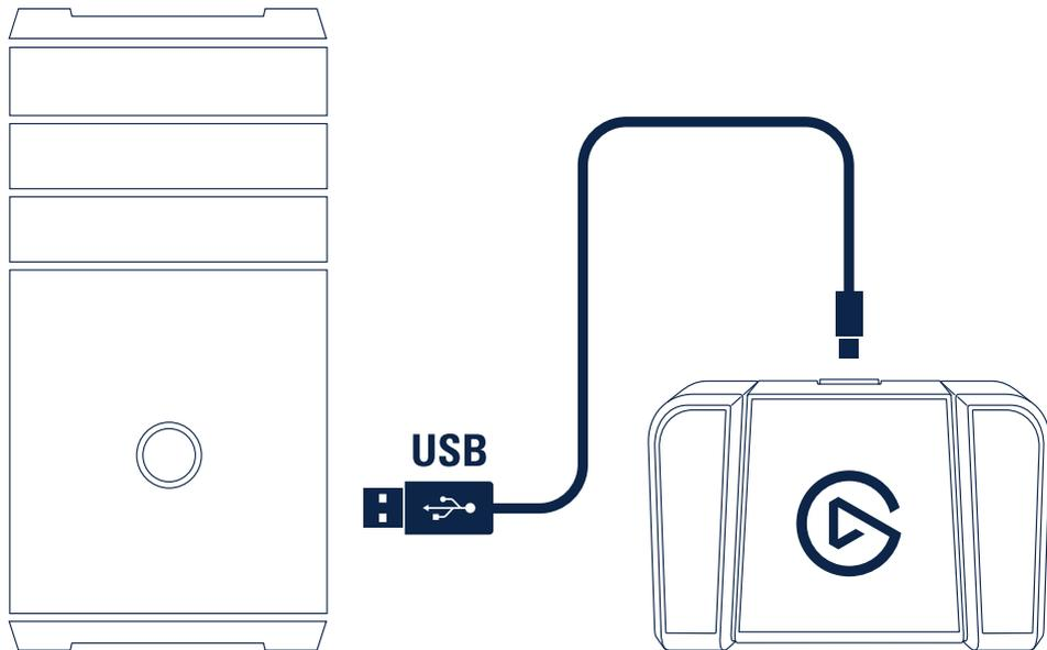
Connect Stream Deck Pedal directly to a USB port on your PC or Mac – do not use a USB hub.
