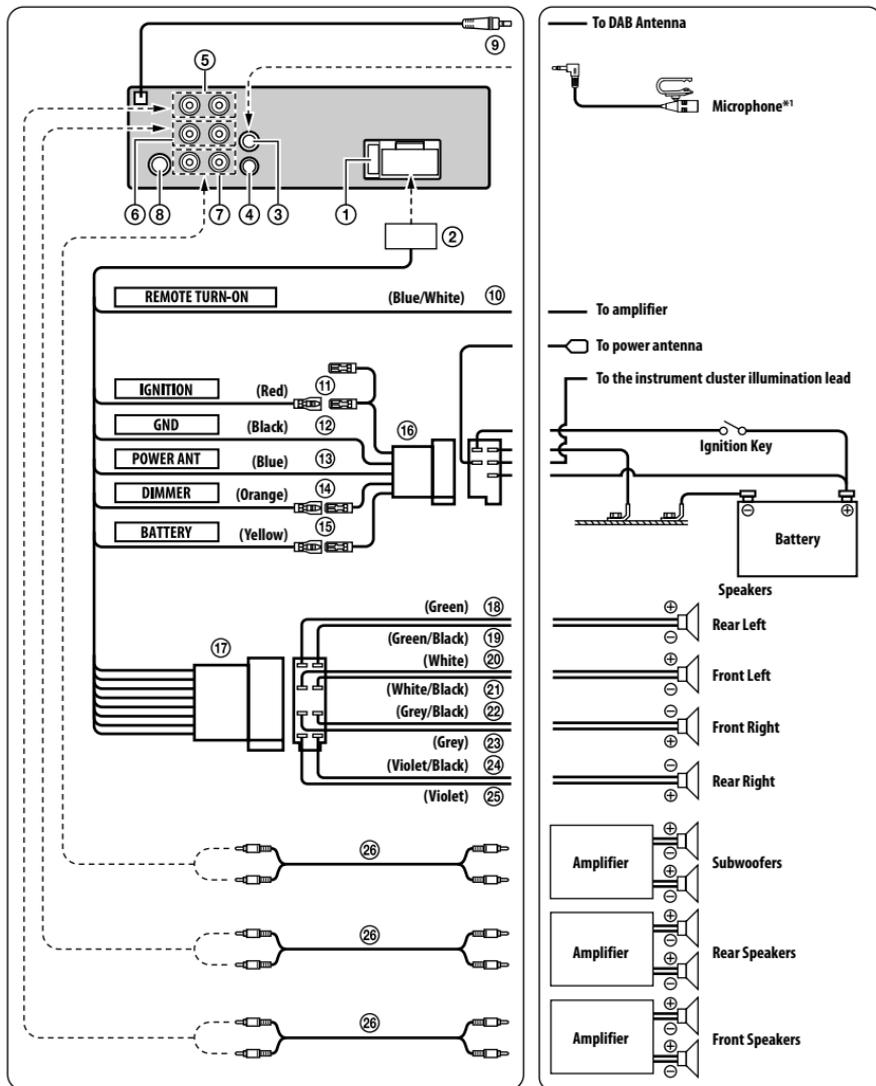
\*1 Whether in use or not, route the microphone input cord such that it does not interfere with driving operations. Secure the cord with a clamp, etc., if it is installed around your feet. For details on installing the microphone, see "Installing the microphone (CDE-205DAB/ UTE-204DAB only)" (page 39).
