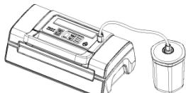
Check the LED status of "vacuumstrength" to confirm the desired vacuum pressure "normal" (normal) or "schonend" (gentle) according to the type of food.
