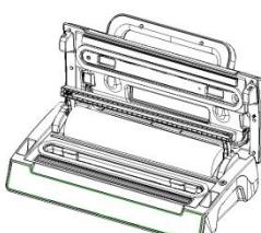
Make sure the bag cutter is on one end of the cutter rack, then put the cutter rack to the back
